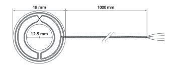
All four ends are tin-plated; the lead ends of the torsion coil are marked black.
